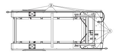
To plug the power cord into an outlet in front of the treadmill, use Hole Pattern 1 for outlets located at the front of the machine.
